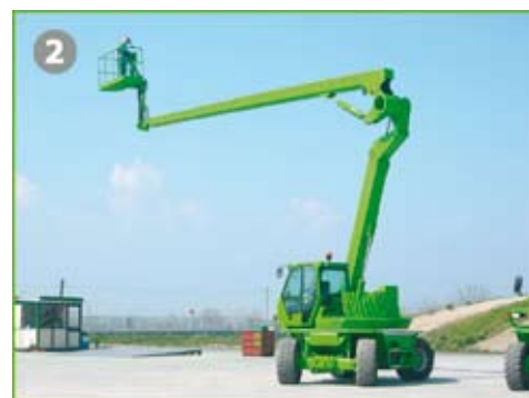
2 Drive the MRP series from the platform at 1km/h even when fully raised (6 km/h when lowered)
