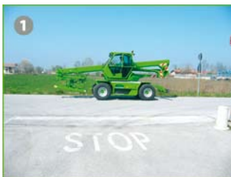
1 Drive the MRP series from the inside the cab at up to 40 km/h for transport
